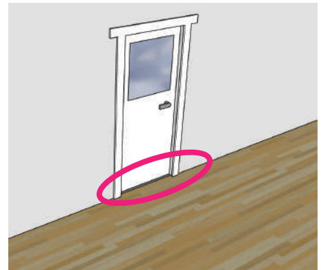
A common exterior doorway to flooring transition
